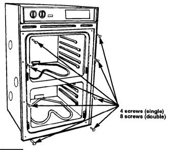
Center oven into cabinet cutout. Use two screws (four screws for a double oven) through the mounting holes in the front frame of the oven to secure the oven to the cabinet. Do Not overtighten screws.
